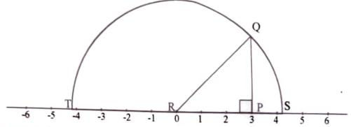
In the figure, a number line is drawn. PQR is a right triangle with PQ = PR. A semicircle is drawn with QR as radius, which cuts the number line at S and T.
